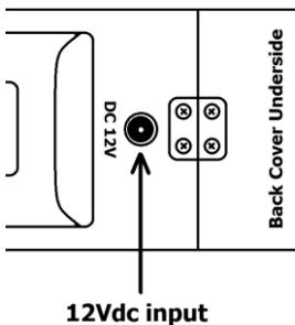
Alternatively, the L25 can be powered by an external 12Vdc source (such as car battery) connected via a 2.1mm DC jack located between the pistol grip and rear cover hinge (a lead is supplied for connection to a car cigar lighter socket). This jack is covered with a rubber plug for protection.
