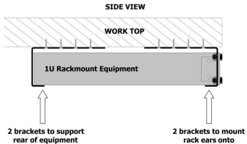
Secure the rack ears through the mounting holes as shown using the supplied screws and hex nuts provided.
