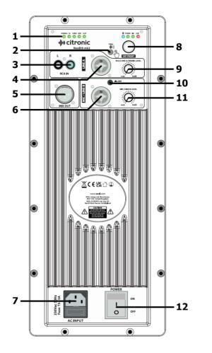
1. DSP setting indicators 2. Bluetooth/TWS pairing button 3. Line A in L+R RCA sockets 4. Line A in combo XLR/jack socket 5. MIX OUT line output XLR 6. Mic/Line B in combo XLR/jack socket 7. IEC mains power inlet and fuse holder 8. DSP preset selector 9. RCA/Line A/Media Level control 10. Input B Mic/Line level switch 11. Mic/Line B / Media Level control 12. POWER on/off switch
