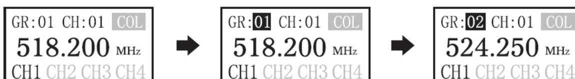
Press the MENU knob once to highlight **GR** and turn the same MENU knob to select from GR1 to GR8, depending on which group of carrier frequencies will be used. Then press the MENU knob again to confirm.
