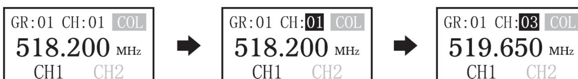
Press the MENU knob three times to highlight **COL** and turn the same MENU knob to select the channel colour, which will be shown in the TFT display and on the backlight for the transmitter LCD screens. Then press the MENU knob again to confirm. (1 channel version shown)
