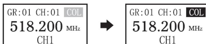
Channel number and channel colour should be set for additional channels on XU2 and XU4 models by pressing the SET button multiple times to navigate to CH1, CH2, CH3, or CH4 tabs at the bottom of the TFT display and repeating the **CH** and **COL** settings described above for each one. (Note: Group is selected for ALL channels and cannot be changed per channel).
