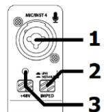
2. IMPED switch Press this button in to set the input impedance to instrument level or leave the button in the up position for a line level input. (instrument level is usually for pickups, such as those on a guitar. Electronic keyboards usually produce a line level output)
