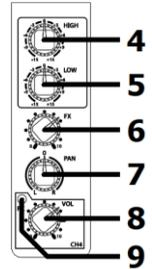
6. FX This control regulates the amount of the channel signal that is fed to the digital delay effects section, varying the amount of delay effect (see Digital Delay below)
