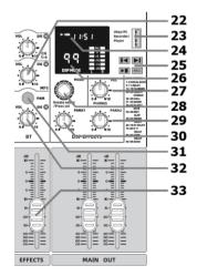
The signal to the PC will be the overall mix of all channels and the signal back from the PC will be added to the main mix via the MP3 volume control.
