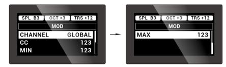
Press SHIFT and MIDI Buttons to enter the MIDI configuration, then push the Modulation Wheel, it will be shown on the screen. Use the five-way encoder to change the parameters.
