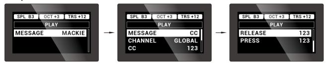
Select DAW Type as USER, then press SHIFT and DAW Buttons to enter the DAW USER Preset configuration. Press any of the Transport Control Buttons (LOOP, STOP, PLAY, RECORD, REWIND, FAST-FORWARD, READ, WRITE), and it will be shown on the screen. Use the five-way encoder to change the parameters.
