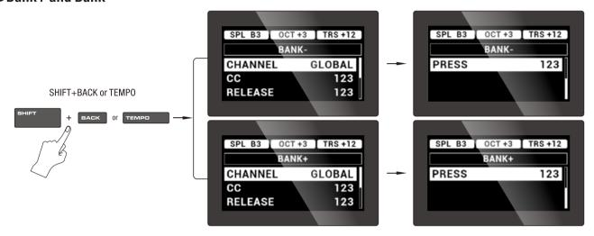
Press SHIFT and MIDI Buttons to enter the MIDI configuration, then press SHIFT and BACK or SHIFT and TEMPO Buttons to configure for Bank- or Bank+. It will be shown on the screen. Use the five-way encoder to change the parameters.
