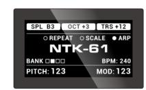
To transpose the keyboard, press and hold the SHIFT Button, then press the OCTAVE Buttons to transpose in semitone steps.
